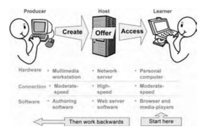
The host requires a network server. You can think of it as an ultra-powerful personal computer optimized for delivering information over a network. The host also needs a high-speed network connection so it can deliver information to many simultaneous learners. And the host requires Web-server software, perhaps including special collaboration tools and media servers.
