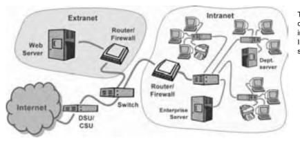
Typical extranet connected to the intranet and the Internet by a shared switch.
