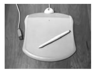
A stylus-tablet that connects to a computer's USB port.
