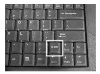
The Sony Vaio Z505 (pictured at left), for example, has a half-sized Shift key on the right side of the keyboard. The lack of a regular sized Shift key frustrates touch typists.
