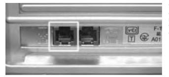
The boxed area on the back of this computer shows the RJ11 port on the modem where the incoming telephone line is connected. You can connect a telephone to the other port.
