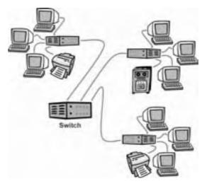
LAN for an organization with several departments. Separate network clusters are connected through a central switch.
