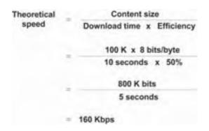
Let's look at an example. Suppose that you want a 100 K Web page to download within 10 seconds over a connection that is 50% efficient. Start by multiplying the 100 K page size by 8 to convert bytes to bits. Then, divide by the target download time of 10 seconds multiplied by the efficiency of 50%.
